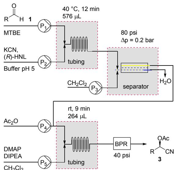
**Scheme 2** Schematic representation of the flow setup
