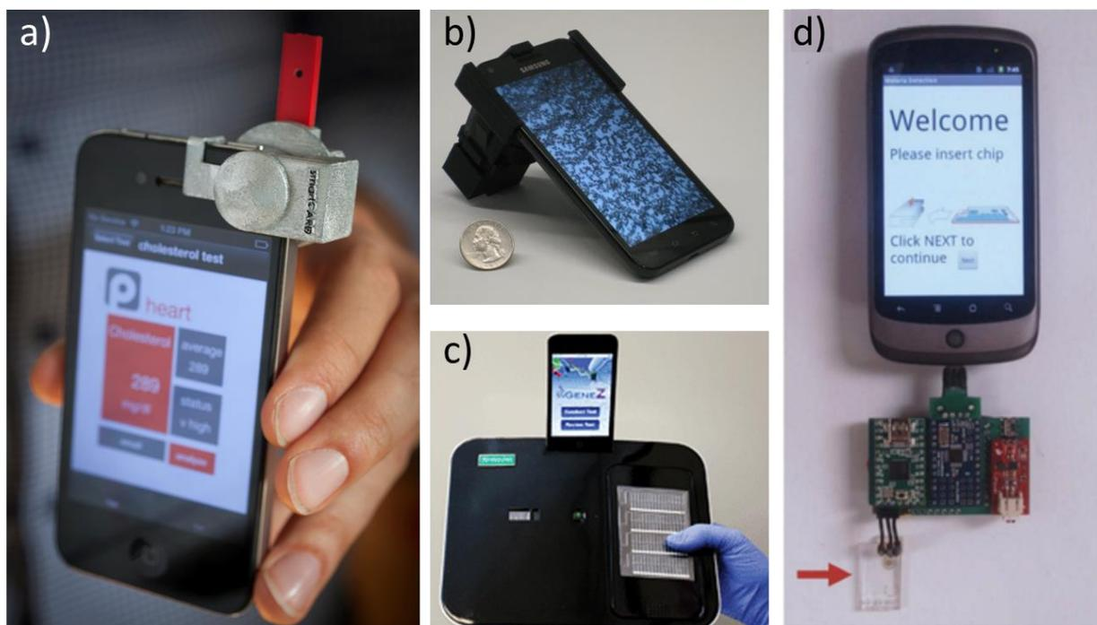
**Figure 1: Smartphone based microfluidic and lab-on-chip technology** (a) colorimetric analysis for serum cholesterol detection [7] (b) smartphone microscopy [8] (c) genetic testing [9] and (d) electrochemistry analysis [10]. Images (b), (c), and (d) Reproduced from [8], [9], and [10] respectively with permission from The Royal Society of Chemistry
