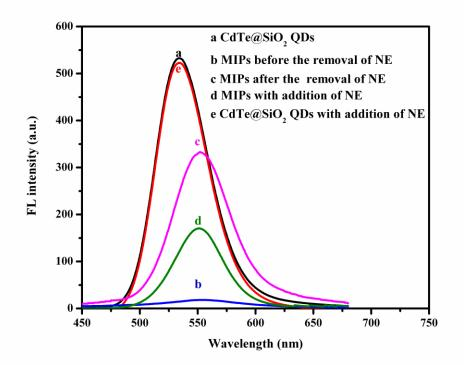
Fig. 7 Fluorescence spectra of CdTe@SiO<sub>2</sub> QDs, CdTe@SiO<sub>2</sub> QDs with addition of NE, CdTe@SiO<sub>2</sub>@MIP before and after the removal of NE and CdTe@SiO<sub>2</sub>@MIP with addition of NE.
