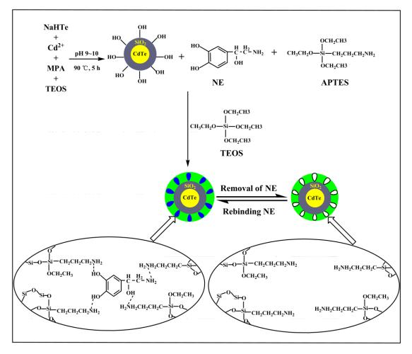
Fig. 1 Schematic illustration of fabricating CdTe@SiO<sub>2</sub>@MIP.
