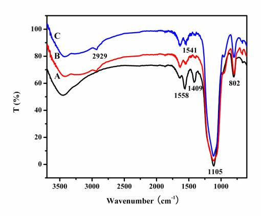
Fig. 2 FT-IR spectra of CdTe@SiO<sub>2</sub> QDs (A), CdTe@SiO<sub>2</sub>@MIP (B) and CdTe@SiO<sub>2</sub>@NIP (C).
