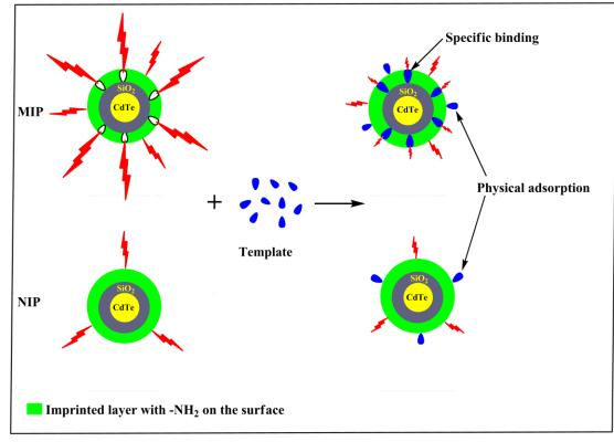
Fig.5 Schematic illustration of the mechanism of interaction between MIP and NIP.
