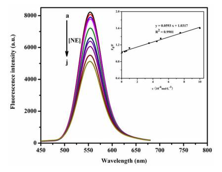
Fig. 6 Fluorescence spectra of CdTe@SiO<sub>2</sub>@MIP at different concentrations of NE and the corresponding Stern-Volmer curve (inset).
