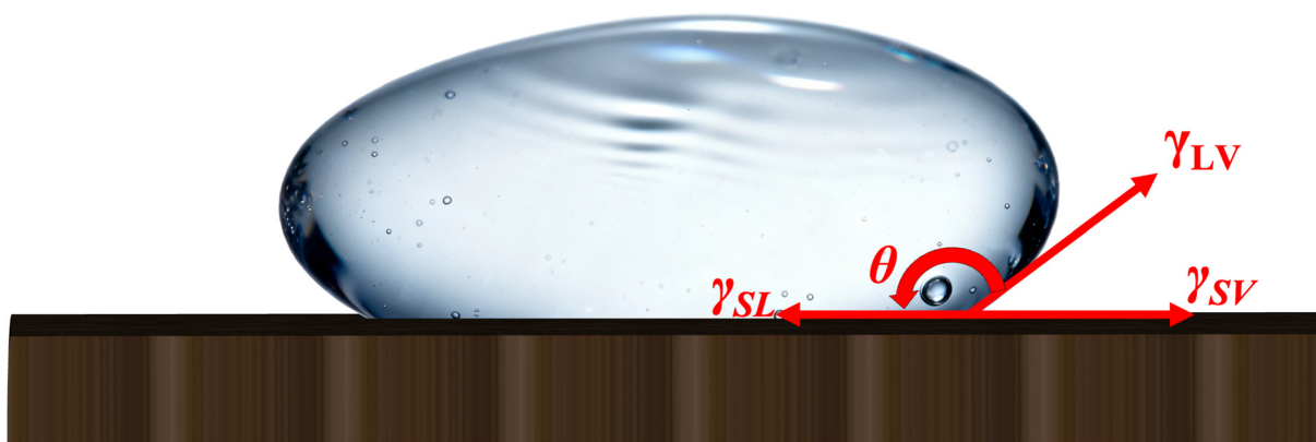
Fig. 4 Three vector components of Young's equation: solid–liquid ( \gamma_{SL} ), solid–vapor ( \gamma_{SV} ), and liquid–vapor ( \gamma_{LV} ) surface tensions. \theta is the contact angle.
