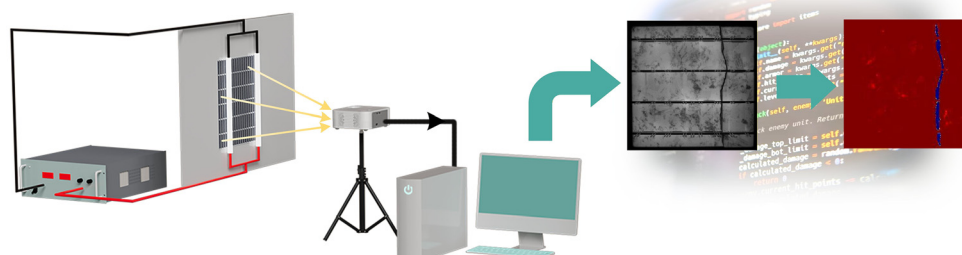
Fig. 1 PVEL image acquisition and machine learning-based defect segmentation.
