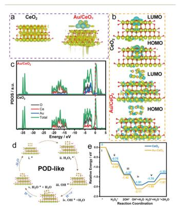
Fig. 5 (a) Charge density difference illustration of  $CeO_2$  and  $Au/CeO_2$ . (b) HOMO-LUMO energy levels and the interfacial diagrams of the molecular orbitals for  $CeO_2$  and  $Au/CeO_2$ . (c) Density of states of  $CeO_2$  and  $Au/CeO_2$ . (d) Proposed reaction pathways of the POD-like reaction. (e) Corresponding free energy diagrams of  $CeO_2$  and  $Au/CeO_2$  for the POD-like reaction.
