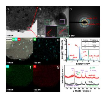
Fig. 2 (a) TEM image of the Au/CeO<sub>2</sub> NB heterostructure. (b) HRTEM images; the rectangular areas represent the FFT patterns of the selected areas (green and purple boxes), (c) SAED pattern of the different areas, and (d) STEM image and the corresponding elemental mapping images of (e) Au, (f) Ce, and (g) O in Au/CeO2. (h) The EDS spectrum and (i) XRD pattern of the Au/CeO<sub>2</sub> heterostructure.
