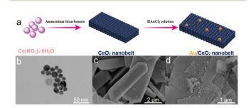
Fig. 1 (a) Schematic illustration of the preparation procedure of the Au/  $CeO_2$  NB heterostructure. SEM images of (b) Au, (c)  $CeO_2$  and (d) Au/  $CeO_2$ .
