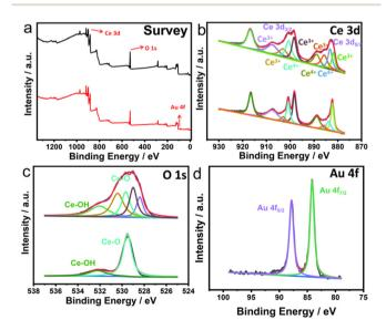
Fig. 3 (a) XPS survey spectra of Au/CeO<sub>2</sub>. The high-resolution XPS spectra of (b) Ce 3d, (c) Au 4f, and (d) O1s of Au/CeO2.
