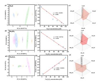
Fig. 7 PCA diagram of the colorimetric sensor array with diverse concentrations of SCMs ((a1) Na<sub>2</sub>S, (a2) Na<sub>2</sub>SO<sub>3</sub> and (a3) Na<sub>2</sub>S<sub>2</sub>O<sub>8</sub>). (b1-b3) Plots of the discriminant factor 1 vs. the concentrations of SCMs. (c1-c3) Radar map of the colorimetric sensor array toward three kinds of SCMs. The y-axis scale represented the absorption intensity of oxTMB in the [Au/CeO<sub>2</sub> + TMB/H<sub>2</sub>O<sub>2</sub>] reaction system.
