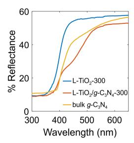
Fig. 5 Diffuse reflectance spectra for lyophilized  $TiO_2$  powder (blue curve) and  $TiO_2/g$ - $C_3N_4$  nanocomposite (red curve) prepared at 300 °C as well as for bulk g- $C_3N_4$  prepared by polymerizing urea at 600 °C (yellow curve).
