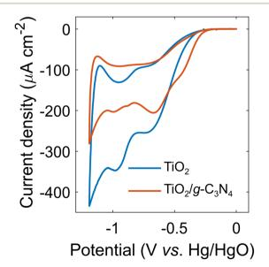
Fig. 7 Cyclic voltammograms for the ORR on the  $TiO_2$  (blue curve) and  $TiO_2/g$ - $C_3N_4$  (red curve) thin films prepared on FTO at 300 °C.
