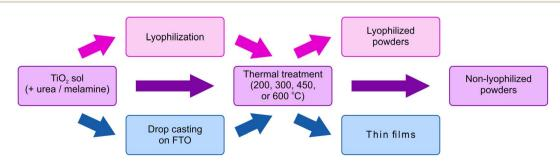
Fig. 2 The synthetic procedure for the preparation of  $TiO_2$  and  $TiO_2/g-C_3N_4$  in the form of non-lyophilized powders, lyophilized powders, and thin films.
