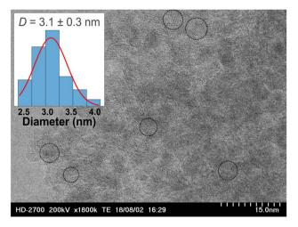
Fig. 1 TEM micrograph of  $TiO_2$  nanoparticles drop-cast from the sol. Several typical particles are marked with dashed circles. The inset shows the corresponding size distribution (blue bars) and the fitting Gaussian function (red curve).
