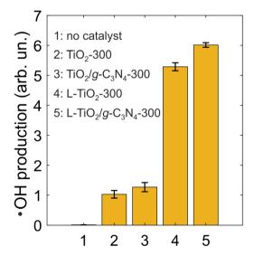
**Fig. 6** \*OH production (as HTA fluorescence intensity) without catalysts and in 1 mg mL $^{-1}$  suspensions of non-lyophilized and lyophilized TiO $_2$  powders and TiO $_2$ /g-C $_3$ N $_4$  composites annealed at 300 °C. The photoactivation was performed with an LED peaking at 385 nm at a light dose density of 36 J cm $^{-2}$  (60 mW cm $^{-2}$  for 10 min).
