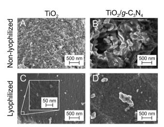
Fig. 4 SEM micrographs for TiO<sub>2</sub> (A) and (C) and TiO<sub>2</sub>/g-C<sub>3</sub>N<sub>4</sub> (B) and (D) samples not subjected (A) and (B) and subjected (C) and (D) to lyophilization before thermal treatment at 300 °C. The images were acquired at a magnification of 50kx. The inset in panel C shows a highresolution image acquired at a magnification of 500k× to resolve the nanoporous structure of this sample
