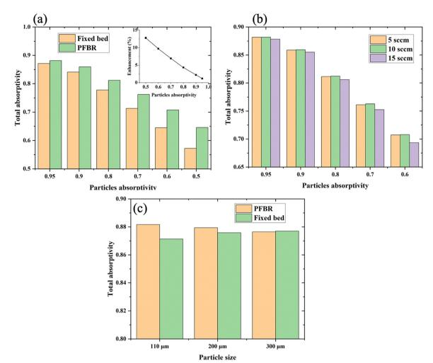
Fig. 4 Comparison of total absorptivity between fluidized bed and fixed bed configurations. (a) Total absorptivity at different particle absorptivities; the inset shows the corresponding enhancement compared to the fixed bed. (b) Total absorptivity at varying gas flow rates. (c) Total absorptivity at different particle sizes (gas flow rate: 5 sccm; particle absorptivity: 0.95). In all cases, the reported absorptivity values represent the time-averaged results over the interval from 0.2 s to 2 s.
