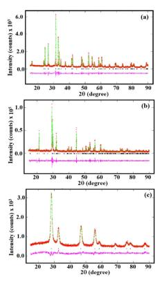
Fig. 1 Lattice refinements of the PXRD patterns of (a) CBOC, (b) CBO, and (c) BCO by the Le Bail method. The red, green, and pink lines are for the experimental data, the calculated, and the difference profiles, respectively.
