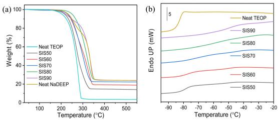
Fig. 2 (a) TGA thermograms of the NaDEEP salt, the TEOP solvent and the SISXX electrolytes, and (b) DSC traces of the SISXX electrolytes and the TEOP solvent
