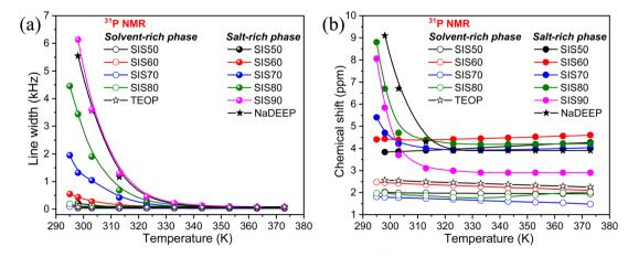
Fig. 7 (a) Line width and (b) chemical shift of 31P NMR spectra of the NaDEEP salt, the TEOP solvent, and the SISXX electrolytes as a function of temperature.
