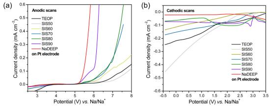
(a) Anodic and (b) cathodic LSV scans of the TEOP solvent, the SISXX electrolytes, and the NaDEEP salt using Pt as the WE
