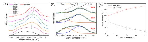
Fig. 5 (a) FT-IR spectra of the NaDEEP salt, the TEOP solvent, and the SISXX electrolytes in the P=O stretching vibrational mode region, (b) deconvolution of this region for SIS50, SIS70 and SIS90, and (c) the resulting peak fractions of "free" P=O and P=O interacting with Na+ (Na+-P=O) as a function of salt content.
