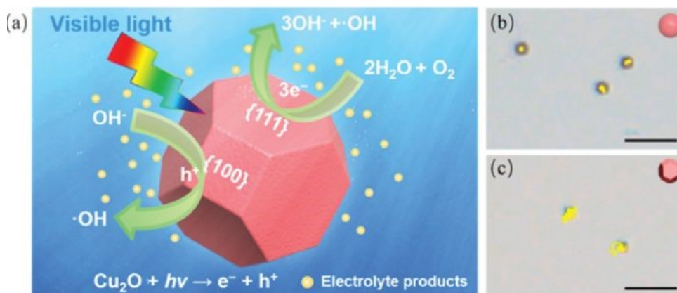
Figure 11. a) Scheme of the propulsion mechanism of a truncated octahedral Vis-LDM based on \text{Cu}_2\text{O} in pure water under visible light irradiation. (b and c) Motion trajectories of spherical (b) and truncated octahedral (c) \text{Cu}_2\text{O} motors over 3 seconds. Scale bar: 5 mm. Reprinted with permission from (36) (Copyright © 2021 Royal Society of Chemistry).
