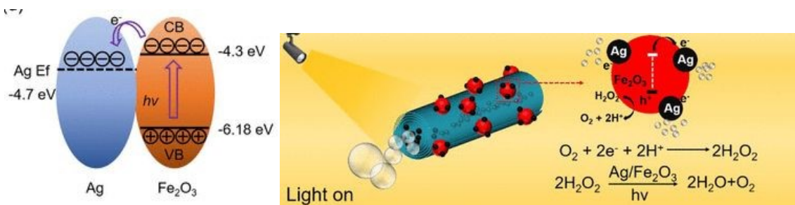
Figure 6. Band structure of the Ag-Fe 2 O 3 heterostructure and schematic illustration of a visible light-enhanced propulsion mechanism. Reprinted with permission from (87) (Copyright © 2022 American Chemical Society).
