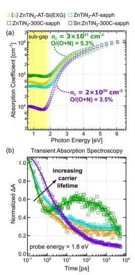
Fig. 4 (a) Absorption coefficient vs. photon energy from spectroscopic ellipsometry for ZnTiN<sub>2</sub> films grown with varying growth conditions. Higher optical quality is indicated by a decrease in the degree of sub-gap (≤2 eV) absorption. (b) Transient absorption kinetics of films grown with varying growth conditions at probe energies of 1.8 eV after photoexcitation at 3.1 eV. Normalized TA kinetic data are shown as markers and fits as solid lines
