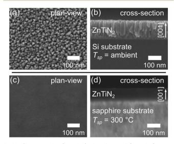
Fig. 2 Representative (a and c) plan-view and (b and d) crosssectional scanning electron microscopy micrographs from a ZnTiN<sub>2</sub>-AT-Si film (top) and a ZnTiN2-300C-sapph film (bottom). Ambient temperature growth on Si produces a polycrystalline (002)-textured columnar microstructure with a rough surface while growth on sapphire at elevated temperature results in a homogeneous and smooth ZnTiN<sub>2</sub> film.
