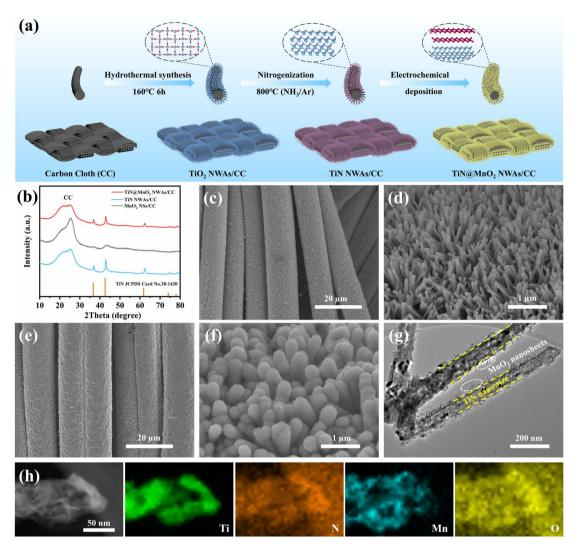
Fig. 2 (a) Schematic diagram of preparation of TiN@MnO $_2$  NWAs/CC. (b) XRD patterns of TiN@MnO $_2$  NWAs/CC, TiN NWAs/CC and MnO $_2$  NSS/CC. SEM images of TiN NWAs/CC (c, d) and TiN@MnO $_2$  NWAs/CC (e, f) at different magnifications. TEM image (g) and EDS element mapping (h) of single TiN@MnO $_2$  nanowires.
