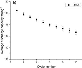
Fig. 8 (a) Galvanostatic charge–discharge profile and (b) average gravimetric discharge capacity against cycle number for LMNO. Cells were cycled at  $10~{\rm m~Ag^{-1}}$  between  $3.5-4.9~{\rm V}$ .
