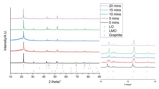
Fig. 3 XRD patterns of 0.3 g end-of-life cathode after leaching in 10 mL of 1 M citric acid for 0 (black), 5 (red), 10 (blue), 15 (green) and 20 minutes (purple) (Co Kα). Tick marks correspond to LO (black), LMO (red) and graphite (blue).
