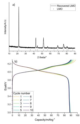
Fig. 6 (a) XRD pattern of recovered LMO (Co Kα) with tick marks correspond to LMO and (b) galvanostatic charge-discharge profile of recovered LMO when cycled at 10 m Ag<sup>-1</sup> between 3-4.3 V.
