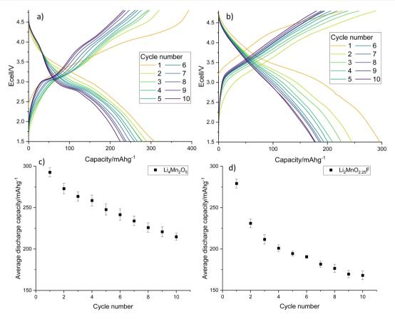
Fig. 10 Galvanostatic charge-discharge profiles for (a) Li<sub>4</sub>Mn<sub>2</sub>O<sub>5</sub> and (b) Li<sub>2</sub>MnO<sub>2.25</sub>F and average gravimetric discharge capacity against cycle number for (c)  $\text{Li}_4\text{Mn}_2\text{O}_5$  and (d)  $\text{Li}_2\text{MnO}_{2.25}\text{F}$ . Cells were cycled at 10 m  $\text{Ag}^{-1}$  between 1.5–4.8 V.
