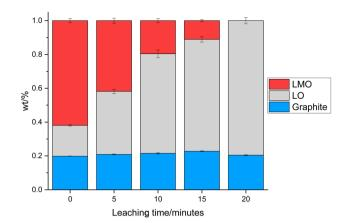
Fig. 4 wt% of LMO (red), LO (grey) and graphite (blue) in the end-oflife cathode at different leaching times from XRD analysis.
