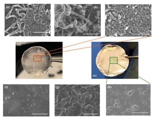
Fig. 1 Scanning electron microscopy (SEM) images of the LMAs at the (a and f) 1st, (b and g) 10th, and (c and h) 100th cycle without (a-c) and with (f-h) Gd(NO<sub>3</sub>)<sub>3</sub> electrolyte additive. Optical images (d and e) show the macroscopic-scale appearance of the respective LMAs after 100 cycles. All SEM images are collected at a scale bar of 20 µm.
