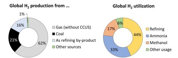
Fig. 2 Production (left) and utilization (right) of  $H_2$  in 2022, according to IEA.<sup>48</sup> "Other sources" in the  $H_2$  production panel include oil (0.5%), fossil fuels coupled to CCUS (0.6%), and water electrolysis (0.1%). "Other usage" in the  $H_2$  utilization panel is mostly linked to the iron and steel industry (DRI, Direct Reduced Iron).
