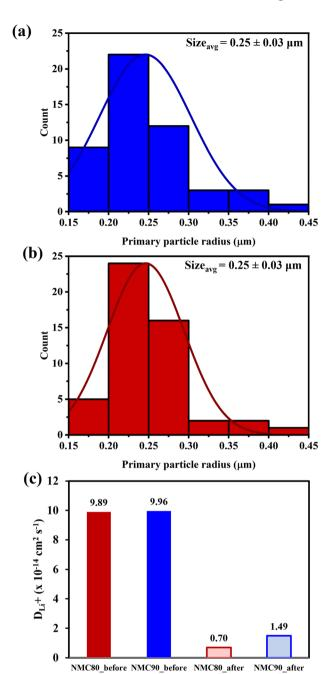
Fig. 6 Primary particle size distribution of the (a) NMC90 and (b) NMC80 powders and (c) the Li<sup>+</sup> diffusion coefficient from the Atlung method for the NMC90 and NMC80 cells before cycling and after cycling.
