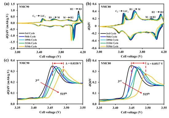
Fig. 4 dQ/dV plots at 0.1C within the voltage range 3.0-4.2 V for the 3rd, 56th, 109th, 212th, and 515th cycles of the (a) NMC90 and (b) NMC80 cells. dQ/dV plots in the  $C_6$  to  $LiC_x$  region of the (c) NMC90 and (d) NMC80 cells.
