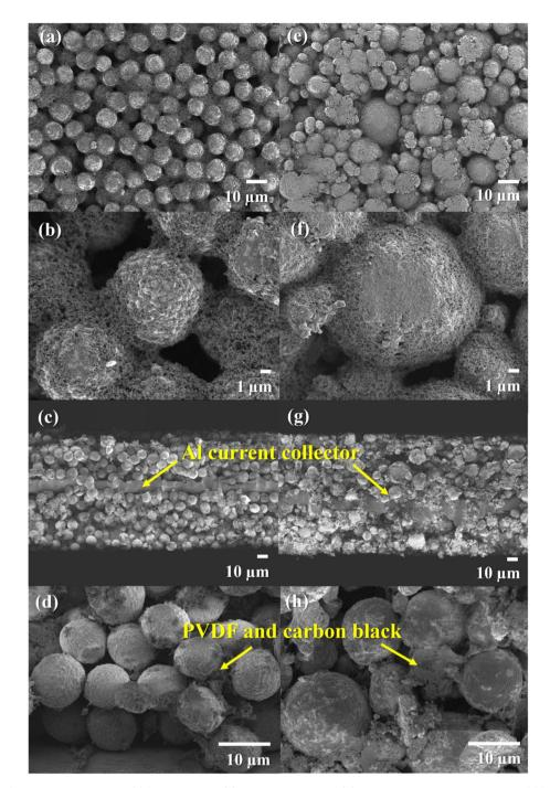
Fig. 2 Top-view FESEM images of the NMC90 electrode at (a) low magnification, (b) high magnification and the NMC80 electrode at (e) low magnification and (f) high magnification, as well as cross-sectional FESEM images of the NMC90 electrode at (c) low magnification, (d) high magnification and the NMC80 electrode at (g) low magnification and (h) high magnification.
