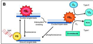
Fig. 1 (A) Simplified mechanism of PDT and SDT. Reprinted with permission from ref. 25. Copyright 2022, Wiley-VCH. (B) Schematic Jablonski's diagram showing the energy transfer and mechanism of action of Type I and Type II pathways in PDT. Reproduced with permission from ref. 26. Copyright 2016, MDPI.
