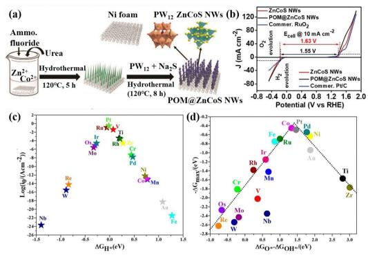
Fig. 4 (a) The synthesis diagram of POM@ZnCoS NWs. (b) Half-cell LSV curves for the OER and HER of the as-prepared electrodes at a scan rate 10 mV s<sup>-1.90</sup> Copyright 2021, Wiley-VCH. (c) HER volcano plot and (d) OER volcano plot of the M<sub>1</sub>/PMA cluster.<sup>91</sup> Copyright 2021, American Chemical Society (ACS).
