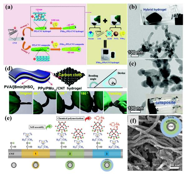
Fig. 19 (a) Fabrication process of PMo<sub>12</sub>/PPy/CNT; TEM images of (b) PMo<sub>12</sub>/PPy/CNT hybrid hydrogel and (c) PMo<sub>12</sub>/PPy/CNT composite. (d) Schematic drawing of the bent SSC and photographs of the flexible SSC under various flexible conditions. 191 Copyright 2020, Royal Society of Chemistry (RSC). (e) Schematic diagram of the synthesis mechanism for 1D coaxial cable-like CNT/PMo/PANI. (f) SEM image of CNT/PMo/PANI. 192 Copyright 2020, Wiley-VCH.
