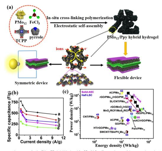
Fig. 22 (a) The preparation process for the PMo<sub>12</sub>/PPy hybrid hydrogel for SCs. (b) Specific capacitances of the prepared samples at various current densities. (c) Ragone plots of the P2-PPy gel//P2-PPy gel device compared with the values reported for other devices. 203 Copyright 2019, Elsevier Ltd.
