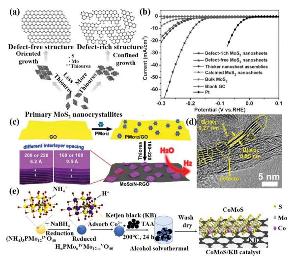
Fig. 9 (a) Structural models and synthetic path diagrams of defect-free and defect-rich structures; (b) LSV curves of various samples as indicated.<sup>126</sup> Copyright 2013, Wiley-VCH. (c) The schematic preparation process of MoS<sub>2</sub>/N-RGO-T nanocomposite; (d) HRTEM of MoS<sub>2</sub>/N-RGO-180. 127 Copyright 2016, Wiley-VCH. (e) Schematic illustration of the synthesis of the CoMoS/KB catalyst. 128 Copyright 2021, American Chemical Society (ACS).
