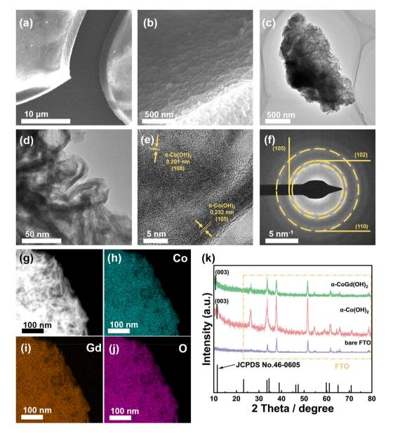
Fig. 2 (a and b) The FESEM images of  $\alpha$ -CoGd(OH)<sub>2</sub>/FTO. (c and d) The TEM images, (e) HRTEM image, and (f) SAED pattern together with the corresponding (g) HAADF pattern as well as the elemental mapping of (h) Co, (i) Gd, and (j) O for  $\alpha$ -CoGd(OH)<sub>2</sub> peeled from the FTO substrate. (k) The powder XRD patterns of bare FTO,  $\alpha$ -Co(OH)<sub>2</sub>/FTO, and  $\alpha$ -CoGd(OH)<sub>2</sub>/FTO.
