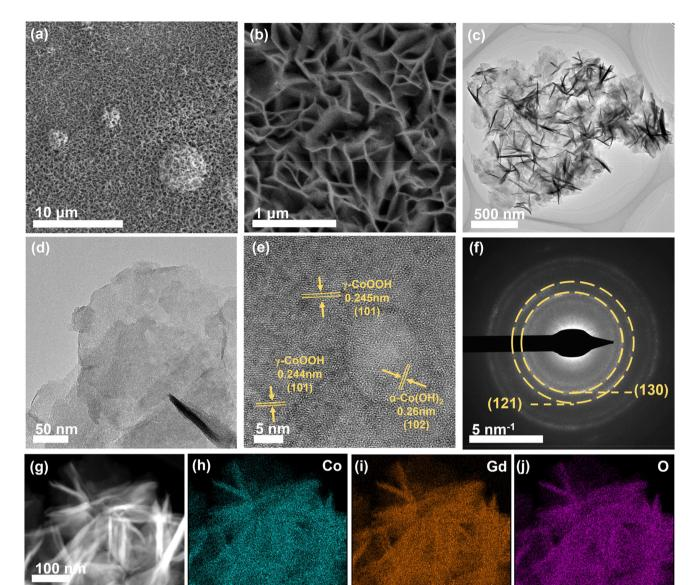
Fig. 4 (a and b) The FESEM images of  $\alpha$ -CoGd(OH)<sub>2</sub>/FTO after activation. (c and d) The TEM images, (e) HRTEM image, and (f) SAED pattern together with the corresponding (g) HAADF pattern as well as the elemental mapping of (h) Co, (i) Gd, and (j) O for  $\alpha$ -CoGd(OH)<sub>2</sub> after activation (peeled from the FTO substrate).
