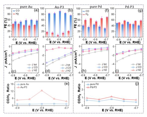
Fig. 2 Electrocatalytic performance for CO<sub>2</sub> reduction: FE and (partial) current density using Au (a and c), Au-P3 (b and d) and the corresponding products ratio (e). FE and (partial) current density using pure Pd (f and h), Pd-P3 (g and i) and the corresponding products ratio (j). A carbon rod was used as a counter electrode and all measurements were carried out in CO2 saturated 0.1 M KHCO3.
