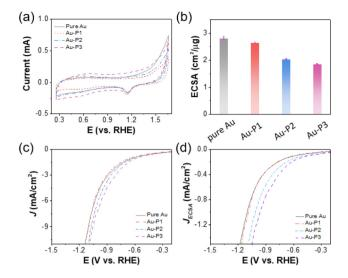
Fig. 1 (a) CV analysis of Au/C modified with fluorinated polymer zwitterions recorded under a scan rate of 100 mV s $^{-1}$  in N<sub>2</sub>-saturated 0.5 M H<sub>2</sub>SO<sub>4</sub>. (b) ECSAs of AuNPs modified with different fluorinated polymer zwitterions. LSV curves measured under a scan rate of 10 mV s $^{-1}$  in CO<sub>2</sub>-saturated 0.1 M KHCO<sub>3</sub> normalized to (c) geometric area of electrodes and (d) ECSA of AuNPs.
