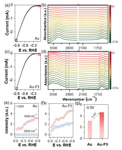
Fig. 3 In situ ATR-SEIRAS study of Au electrodes modified with different fluorinated polymer zwitterions. LSV scans in CO<sub>2</sub> saturated 0.1 M KHCO<sub>3</sub> and in situ ATR-SEIRAS spectra obtained in the range from 0 to -0.9 V for Au (a and b) and Au-P3 (c and d). Peak intensity study for AuNPs (e) and Au-P3 (f) with various reductive potentials. (g) O-H bending model at 1648 cm<sup>-1</sup> under -0.9 V.
