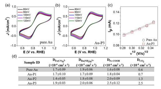
Fig. 5 Mass transport properties of all catalysts. (a) CV scans of AuNPs and (b) Au-P3 measured with 5 mM K₃Fe(CN)<sub>6</sub> under various scan rates. (c) Linear relationship between peak current  $(I_p)$  and the square root of scan rates for pure Au and Au-P3. (d) Summary of diffusion coefficient (D) using various probe molecules including Fe(CN)<sub>6</sub><sup>3-</sup>, Ru(NH<sub>3</sub>)<sub>6</sub><sup>3+</sup>, Fc-COOH, and CO<sub>2</sub>.
