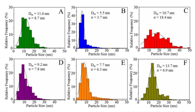
Fig. 9 Particle-size distribution histograms of reduced mono- and bimetallic catalysts: (A) Ni/S, (B) Pd/S, (C) Pt/S, (D) NiPd/S, (E) NiPt/S, and (F) PdPt/S.
