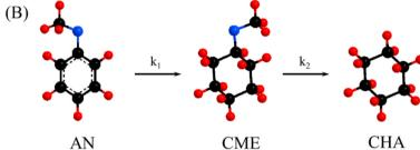
Scheme 1 (A) Proposed reaction mechanism for the hydrodeoxygenation of anisole with prepared mono- and bimetallic catalysts. (B) Simplified reaction mechanism used for the kinetic study. AN, anisole; BEN, benzene; CME, cyclohexyl methyl ether; CHL, cyclohexanol; CHE, cyclohexene and CHA, cyclohexane.
