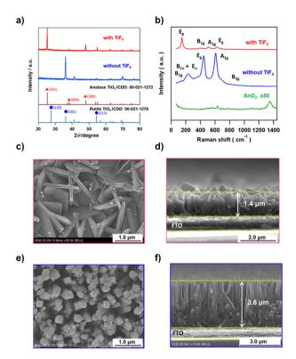
Fig. 1 XRD patterns (a) and Raman spectra (b) of the samples hydrothermally synthesized without and with  $TiF_4$ . Top view (c) and side view (d) SEM images of the DP-Au/A- $TiO_2$  NPLA. Top view (e) and side view (f) SEM images of the DP-Au/R- $TiO_2$  NWA.
