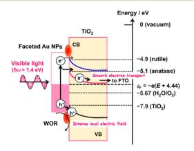
Fig. 5 Action mechanism of the DP-Au/A-TiO $_2$  NPLA and DP-Au/R-TiO $_2$  NWA plasmonic electrodes for the WOR.
