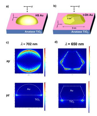
Fig. 4 Local electric fields for HS-Au/A-TiO<sub>2</sub> (a) and t-Oh-Au/A-TiO<sub>2</sub> (b) calculated by the 3D-FDTD method. Local electric field distributions in HS-Au/A-TiO2 (c) and t-Oh-Au/A-TiO2 (d).
