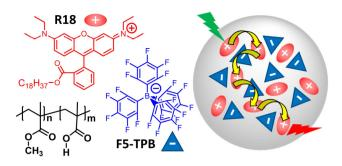
**Fig. 1** Chemical structures of dye (R18) with its bulky counter ion (F5-TPB) and polymer (PMMA-MA) constituting dye-loaded polymeric, light-harvesting nanoparticles sketched on the right-hand side.
