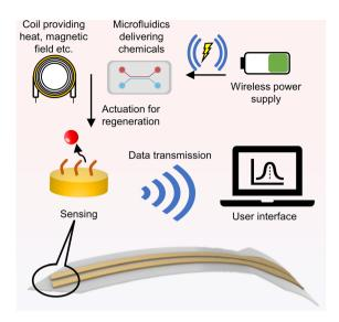
Fig. 7 Schematic illustration of a proposed regeneratable *in vivo* biosensor for real-time monitoring, as discussed in this mini-review. The integration of sensing and actuation elements will facilitate the dissociation of analytes from the device upon an external stimulus transmitted to the system wirelessly.
