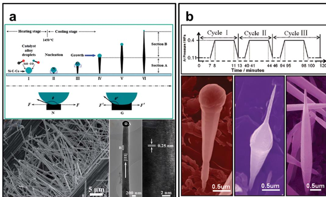
**Fig. 7** (a) Controlled growth of quiasligned SiC nanoarrays with clear and sharp tips. Reprinted with permission from ref. 125. Copyright 2014 by Royal Society of Chemistry; (b) manipulate and control the morphology of SiC nanowires by varying the pressure of the source species. Reprinted with permission from ref. 126. Copyright 2008 by Royal Society of Chemistry.
