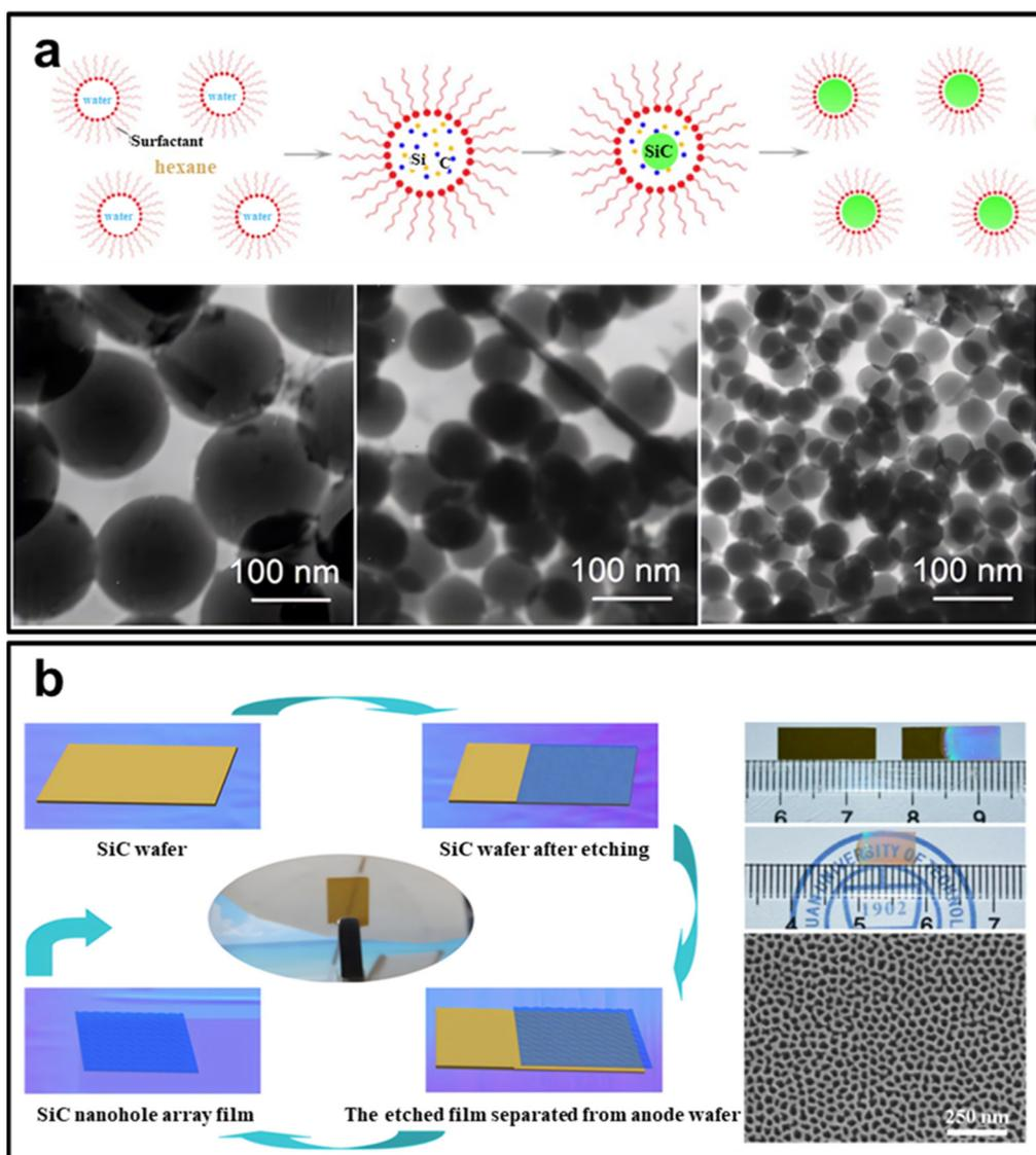
**Fig. 9** (a) The morphology and size of SiC nanospheres synthesized with varying hexane/water volume ratio. Reprinted with permission from ref. 138. Copyright 2017 by Elsevier and Copyright Clearance Center; (b) large-scale fabrication of free-standing and transparent SiC nanohole array with tailored structures. Reprinted with permission from ref. 143. Copyright 2018 by Elsevier and Copyright Clearance Center.
