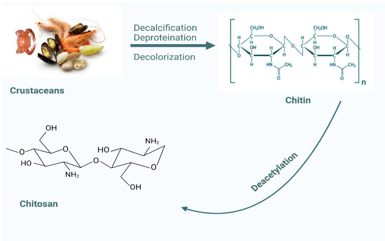
Fig. 3 Process of chitosan extraction.
