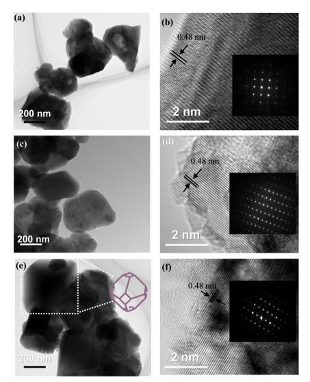
Fig. 4 HR-TEM images of (a) and (b) LMO, (c) and (d) LMTO, and (d) and (f) LMTOS (scale bar: 200 nm and 2 nm), and the inset shows the corresponding SAED pattern (region shown in (b) LMO, (d) LMTO and (f) LMTOS particles).
