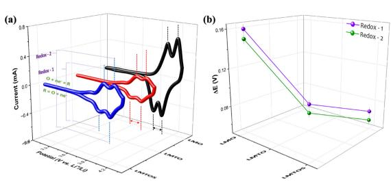
Fig. 7 (a) CV results of the cathodes, with experiments conducted at a scan rate of 0.2 mV s<sup>-1</sup> within a potential range of 3.1–4.3 V. (b) CV redox peak potential difference  $(\Delta E_p)$  for three cathode configurations, emphasizing distinct redox peaks.
