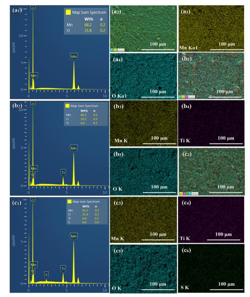
Fig. 2 FE-SEM with EDS results of (a1) LMO, (b1) LMTO, and (c1) LMTOS particles. EDS mapping results: (a1) LMO, (b1) LMTO, and (c1) LMTOS (Mn ((a2), (b2), and (c2)); Ti ((b3) and (c3)); O ((a3), (b4); and (c4)); and S (c5)).
