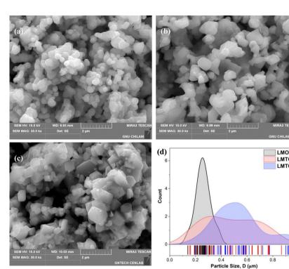
Fig. 3 FE-SEM surface images of (a) LMO, (b) LMTO, (c) LMTOS particles (scale bar in all images: 2 µm), and (d) particle-size distribution for three synthesized particles. LMO, LMTO, and LMTOS are depicted by the black, red, and blue curves, respectively.
