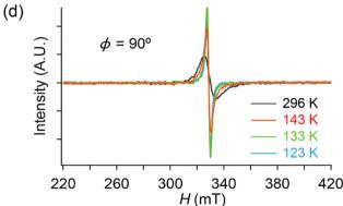
Fig. 5 Comparison of the T-dependent ESR spectra between different orientations ( $\theta$ ,  $\phi$  = 0 and 90°) and between different rotation axes (b- and c-axes) of  $\alpha\text{-ET}_2I_3.$  The sample (single crystal) was rotated around the baxis (a), (b) and the c-axis (c), (d) with the indicated magnetic-field-angle  $\theta$ and  $\phi$ , respectively.  $\boldsymbol{H} \| \boldsymbol{a}$ -axis when  $\theta = 0^{\circ}$  and  $\phi = 0^{\circ}$ .
