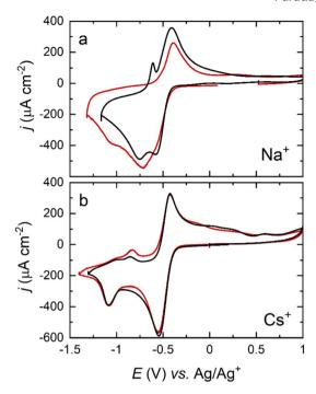
Fig. 6 Cyclic voltammograms of a Pt(111) (black) and a Pt(100) (red) electrode in an  $O_2$ -saturated DMSO solution containing (a) 0.1 M NaClO<sub>4</sub> and (b) 0.1 M CsClO<sub>4</sub>. Scan rate: 50 mV s<sup>-1</sup>.
