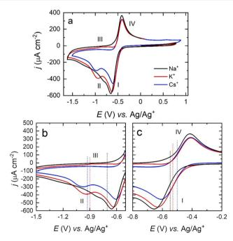
Fig. 5 (a) Cyclic voltammograms of a Pt(poly) electrode in an  $O_2$ -saturated DMSO solution containing 0.1 M NaClO<sub>4</sub> (black), KClO<sub>4</sub> (red) and CsClO<sub>4</sub> (blue), at 50 mV s<sup>-1</sup> scan rate. Expanded view of the potential range corresponding to the formation of  $O_2^{-2}$  (b) and  $O_2^{-1}$  (c). Dotted lines represent the  $E_{1/2}$  of the ORR half reactions for Na<sup>+</sup> (black), K<sup>+</sup> (red) and Cs<sup>+</sup> (blue).
