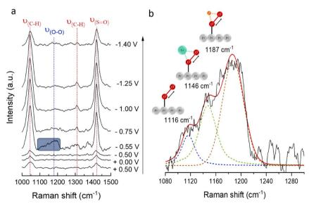
Fig. 7 (a) Potential-dependent in situ SHINERS spectra obtained from a Pt(111) electrode in a solution containing 0.1 M CsClO<sub>4</sub>/DMSO, purged with Ar and, subsequently, saturated with O<sub>2</sub>. (b) Voigt model fitting of  $\nu_{\rm (O-O)}$  at -0.55 V.
