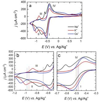
Fig. 4 (a) Cyclic voltammograms of a Pt(111) electrode in an  $O_2$ -saturated DMSO solution containing 0.1 M NaClO<sub>4</sub> (black), KClO<sub>4</sub> (red) and CsClO<sub>4</sub> (blue). Scan rate: 50 mV s<sup>-1</sup>. Expanded view of the peaks relating to the formation of  $O_2^{-1}$  (b) and  $O_2^{-1}$  (c). Dotted lines represent the calculated  $E_{1/2}$  of the ORR half reactions for Na<sup>+</sup> (black), K<sup>+</sup> (red) and Cs<sup>+</sup> (blue).
