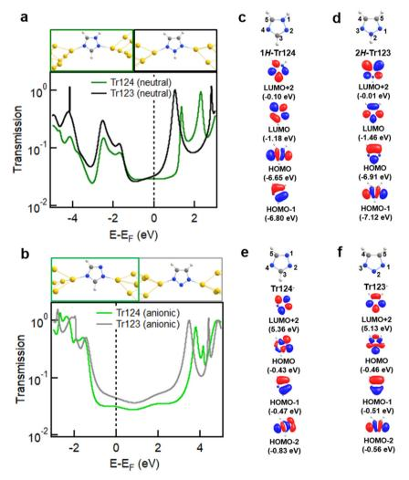
Fig. 4 (a, b) Relaxed junction geometries with neutral and anionic Tr124 and Tr123 bound between two Au18 pyramids with the apex Au-Au distance corresponding to potential energy minimum (top) and the calculated transmission spectra (bottom). Frontier MOs of Tr124 and Tr123 in neutral (c, d) and anionic (e, f) forms and calculated using FHI-aims package with a "tight" basis set and the PBE functional (see Fig. S6 and S7† for the complete pictures of MO plotting).
