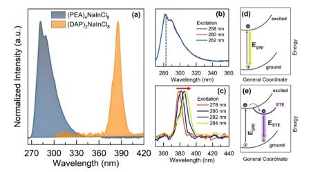
Fig. 3 (a) Normalized PL-intensity of two-dimensional double perovskites; excitation-dependent photoluminescence spectra (PLE) for: (PEA)<sub>4</sub>NaInCl<sub>8</sub> and (DAP)<sub>2</sub>NaInCl<sub>8</sub>, (b) and (c) respectively. Schematic sketch of radiative recombination in the 2D-RP structure (d) and 2D-DJ structure (e).
