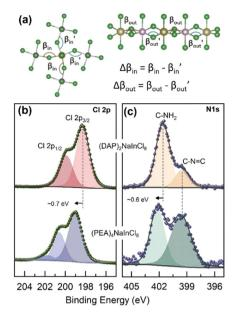
Fig. 2 (a) Schematic showing the asymmetric in-plane and out-of-plane tilting within the inorganic parts of the perovskites along with their mathematical definitions used to build Table 1. XPS core-level spectra of (b) Cl 2p and (c) N 1s of the 2D perovskite (DAP)<sub>2</sub>NaInCl<sub>8</sub> (upper panel) and (PEA)<sub>4</sub>NaInCl<sub>8</sub> (lower panel).
