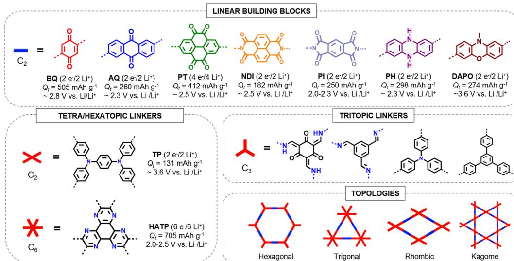
Fig. 5 Library of some representative electroactive organic building blocks (theoretical capacities and average discharge voltages), linkers and topologies used for the synthesis of redox-active COF cathodes in LIBs. BQ (benzoquinone), AQ (anthraquinone), PT (pyrene-tetraone), NDI (naphthalene diimide), PI (polyimide), PH (phenazine), DAPO (phenoxazine), TP (tetraphenyl-*p*-phenylenediamine), and HATP (hexaazatriphenylene).
