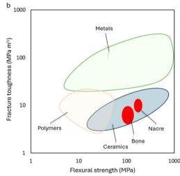
Fig. 5 Exploring material strength: Ashby plot contrasts the mechanical properties of diverse materials with those of bone and nacre, offering insights into the relative performance and suitability for various engineering applications. (a) Compressive strength based on Young's modulus, (b) fracture toughness is based on Flexural strength. The data extracted from ref. 27, 29, 64–69.
