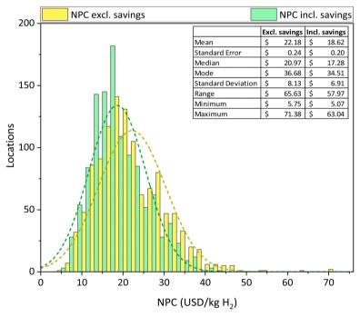
Fig. 5 Histograms of the NPC of  $H_{2,g}$  "today", excluding (yellow) and including (green) the potential savings from the sale of surplus electricity. The sale of this electricity would result in an average saving of 11% on the NPC of green  $H_2$ .
