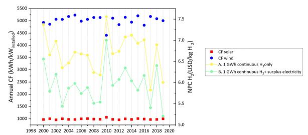
Fig. 8 Cost of intermittency. The annual NPC of green  $H_2$ , excluding (yellow) and including (green) the potential savings from the sale of surplus electricity, together with wind and solar energy CFs over the last 20 years (2000–2019), are displayed for the Isle of Jura in the UK (Lat: 56, Lon: -6).
