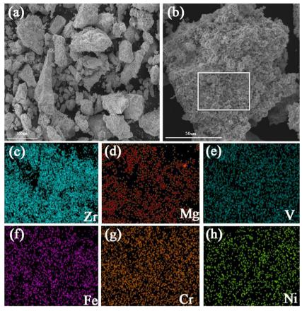
Fig. 3 SEM images (a) and (b) and EDS mappings (c)–(h) of the Zr<sub>2</sub>MgVFeCrNi high-entropy alloys.
