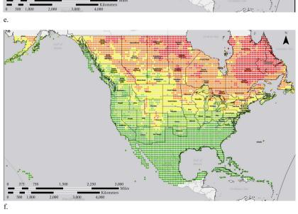
Fig. 3 The percent change in PV potential lost due to snow cover for the optimistic SSP126 scenarios between 2019 and the modeled years of (a) 2040, (b) 2080 and (c) 2100 and the pessimistic SSP585 scenario for (d) 2040, (e) 2080 and (f) 2100.
