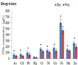
Fig. 2 Trace element concentration ( $\mu$ g L<sup>-1</sup>) in surface and deep water samples of Buriganga River in Bangladesh. "\*" indicates a statistically significant difference in TEs between the dry and wet seasons.
