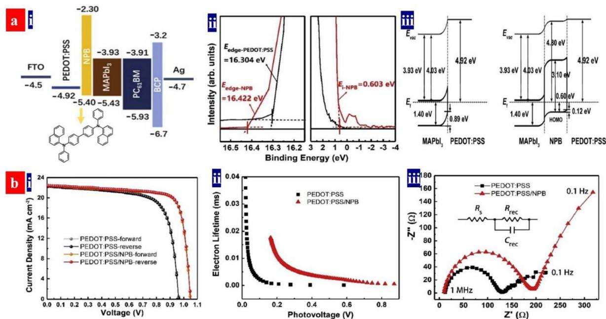
Fig. 10 (a) (i) Energy level diagram and molecular structure of NPB; (ii) UPS of the PEDOT:PSS HTLs; and (iii) energy level alignment diagrams at PEDOT:PSS/MAPbI<sub>3</sub> and PEDOT:PSS/NPB/MAPbI<sub>3</sub> interfaces. (b) (i)  $J$ - $V$  curves of the inverted PSCs; (ii) extracted lifetime of the injected carriers versus photovoltage; and (iii) electrical impedance spectroscopy spectra. Reproduced with permission.<sup>143</sup> Copyright 2022, Elsevier.
