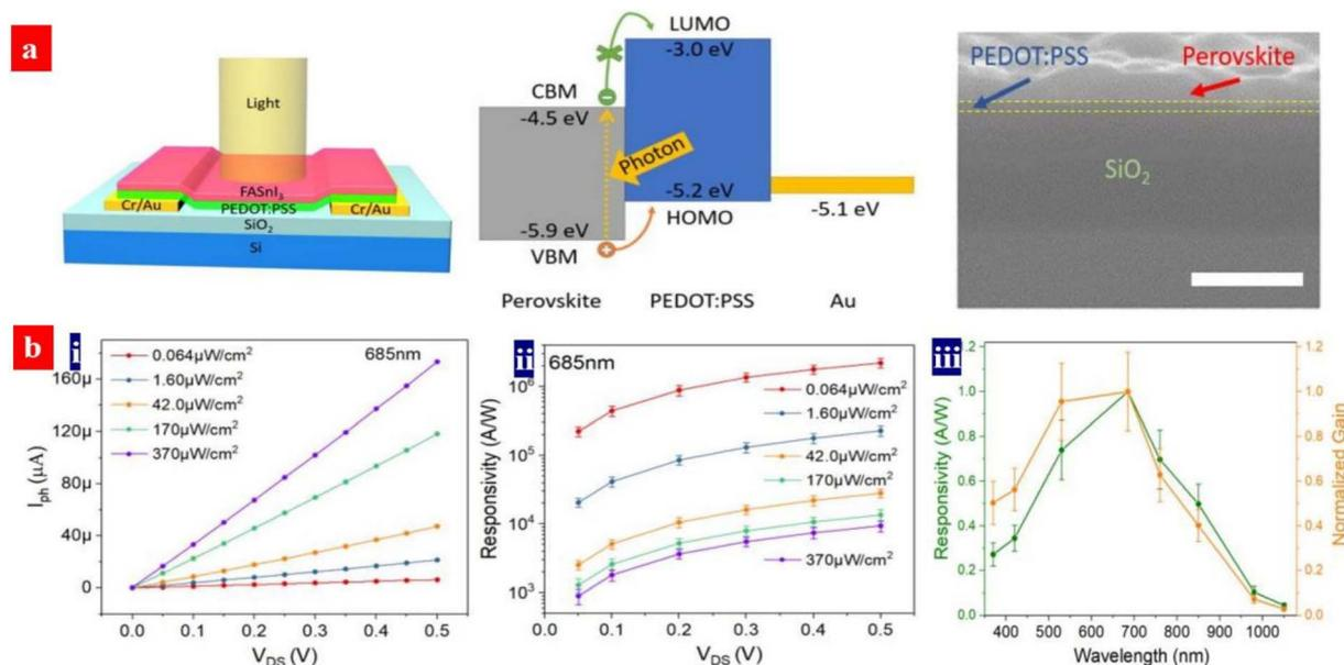
Fig. 11 (a) Architecture structure of the PDs, energy band diagram, and cross-sectional SEM image of (a) FASnI<sub>3</sub>/PEDOT:PSS bilayer coated on SiO<sub>2</sub>/Si. Scale bar: 300 nm. (b) (i) Photo-current vs. drain voltage; (ii) average responsivity vs. drain voltage under various intensity of light. Wavelength: 685 nm; and (iii) normalized spectral responsivity and gain of the PD. Reproduced with permission.<sup>157</sup> Copyright 2020, American Chemical Society.
