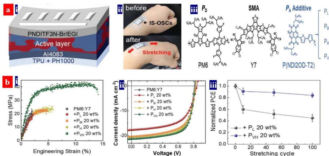
Fig. 20 (a) (i) Stretchable OSC structure, (ii) photographs, and (iii) molecular structures of the PA additives. (b) (i) Stress–strain curves of PM6:Y7 with 20 wt% of PAs of different  $M_w$ s, (ii)  $J$ - $V$  curves of the stretchable OSCs as functions of PAs with different  $M_w$ , and (iii) normalized PCE curves of the stretchable devices in the flexing tests. Reproduced with permission.<sup>199</sup> Copyright 2022, Wiley-VCH.
