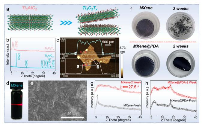
Fig. 3 (a) Illustration of MXene synthesis. (b) XRD characterization of the obtained MXene. (c) AFM characterization of the obtained MXene. (d) Tyndall effect of the obtained MXene dispersion. (e) The surface of the MXene@PDA layer. (f) Digital photos and (g) XRD patterns of MXene-Fresh and MXene-2W. (h) XRD patterns of MXene@PDA-Fresh and MXene@PDA-2W films.
