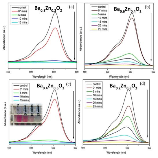
Fig. 7 Influence of Zn doping on the photocatalytic degradation of RhB using (a)  $Ba_{0.8}Zn_{0.2}O_2$ , (b)  $Ba_{0.6}Zn_{0.4}O_2$ , (c)  $Ba_{0.4}Zn_{0.6}O_2$  and (d)  $Ba_{0.2}Zn_{0.8}O_2$  photocatalysts under UV light irradiation.
