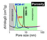
Fig. 2 A comparison of the XRD and pore size distribution of bioinspired silica with two archetypal ordered mesoporous silica materials, SBA-15 and MCM-41. Part of this figure is reproduced with permission from ACS Publications.<sup>28</sup>
