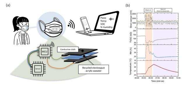
Fig. 6 (a) Conceptual schematic illustrating the potential application and implementation of recycled acrylic materials for piezoelectric sensing. (b) Raw data from a one-minute use of a clothe mask outfitted with the electronic textile made from recycled acrylic sweater and a Bosch RMF680 sensor
