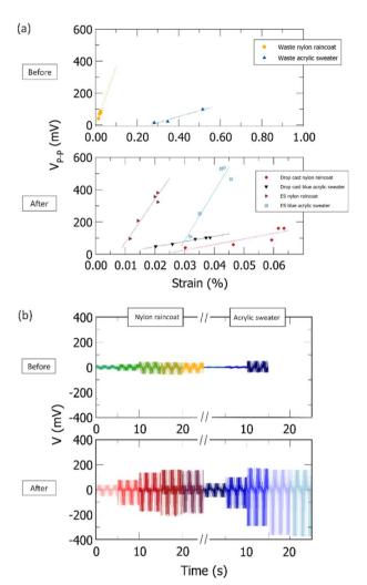
Fig. 4 Each second-hand textile, before (top) and after (bottom) processing and electrospinning, was studied using a cantilever device. (a) The output voltage as a function of strain for each comparable material was linearly fit. (b) The raw output voltage at various strain intensities, where green to yellow and red curves are the nylon material and blue curves are acrylic materials.
