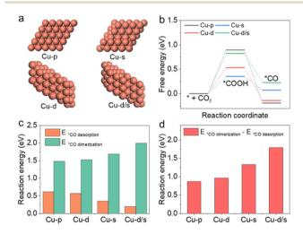
Fig. 4 (a) DFT periodic slab models for Cu(111)-pristine, Cu(111)dislocation, Cu(111)-step and Cu(111)-dislocation/step structures (denoted as Cu-p, Cu-d, Cu-s and Cu-ds, respectively). (b) Gibbs freeenergy diagrams for the proposed steps of conversion of CO<sub>2</sub> to \*CO intermediate. (c) Reaction energies for \*CO desorption to CO and \*CO coupling to \*OCCO on Cu catalysts with various defects. (d) Differences in reaction energies for \*CO coupling to \*OCCO and \*CO desorption to CO
