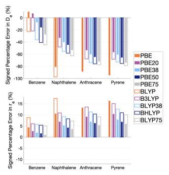
Fig. 5 Percentage error in dissociation energy ( $D_{\rm e}$ , top) and equilibrium inter-monomer separation ( $r_{\rm e}$ , bottom) of each excimer with respect to SCS-CC2/CBS(3,4) for varied Fock exchange with PBE and BLYP exchange-correlation functionals. BLYP results are not shown for anthracene and pyrene excimers as they gave repulsive dissociation curves.
