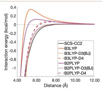
Fig. 12 Unphysical repulsive region for the benzene excimer state dissociation curve and its correction by ground-state optimised dispersion corrections.
