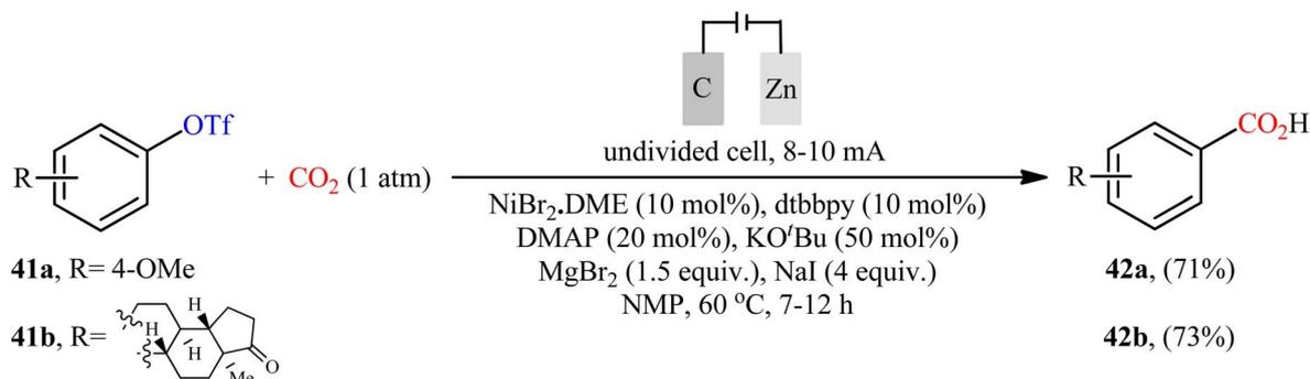
Scheme 23 Electrochemical carboxylation of aryl triflates **41** with CO<sub>2</sub>.
