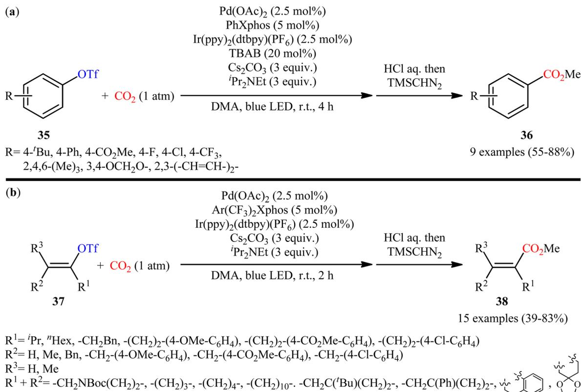
Scheme 20 (a) Metallaphotoredox-catalyzed carboxylation of aryl triflates **31** and (b) alkenyl triflates **33** with atmospheric  $\text{CO}_2$ .
