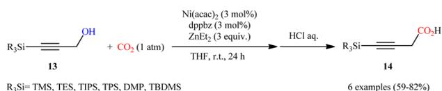
Scheme 8 Ni-catalyzed carboxylation of propargylic alcohols **13** with CO<sub>2</sub>.
