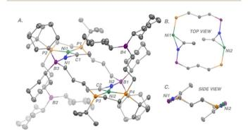
Fig. 3 (A) Molecular structure of 2; (B) top view; (C) side view. Thermal ellipsoids are shown at the 50% probability level. Hydrogen atoms have been omitted for clarity. Selected bond distances (Å): N1–C1 1.236(2), N2–C2 1.236(2), Ni1–Ni2 6.484(8), B1–N2 1.629(2), B3–N1 1.629(2), Ni1–N1 1.907(14), Ni2–N2 1.907(14), Ni1–C1 1.856(17), Ni2–C2 1.856(17).
