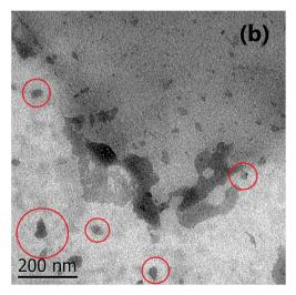
Fig. 7 TEM images from (a) D1-t: the red squares inside the micrography enclose the accumulated GQD very close between them and (b) ZD1-t: the red circles enclose the ZnNP which are mostly lesser than 100 nm.
