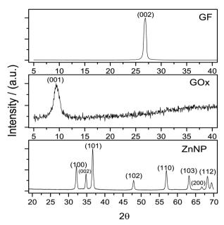
Fig. 1 Normalized XRD diffraction patterns from graphite (GF), graphene oxide (GOx) and zinc nanoparticles (ZnNP). Graphite has a characteristic peak at  $2\theta=26^\circ$  whilst the GOx presents its peak at  $2\theta=10^\circ$ . XRD pattern from ZnNP exhibited characteristic peaks at the angles  $2\theta=31$ , 34, 36, 47, 56, 62, 66, 68 and 69°.
