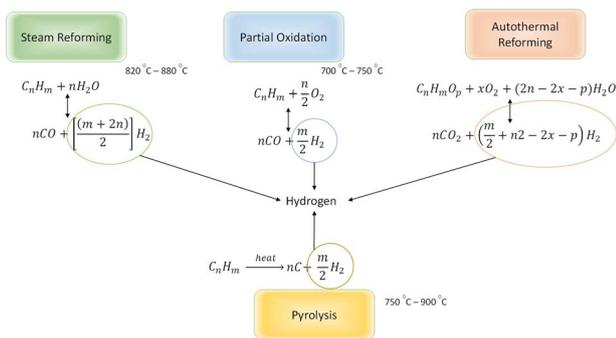
Fig. 2 Summary of hydrogen forming reactions for hydrocarbons.
