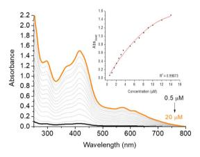
Fig. 3 UV-vis aggregation assays of corrole H<sub>3</sub>LapCor in DMSO(5%)/ Tris-HCl pH 7.4 buffer mixture solution, in the concentration variation from 0.5 to 20  $\mu$ M. Inset: Abs<sub>Soret</sub> versus concentration plot.
